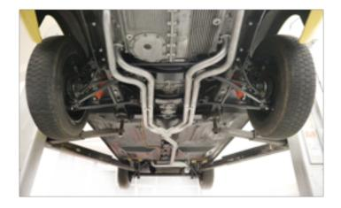
The car comes with it's complete new original exhaust system with an extra pipe replacing the end silencer for a more sporty sound.
