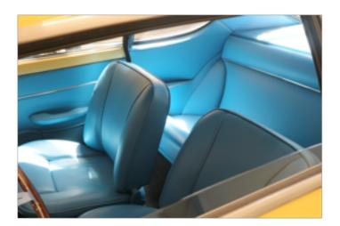
The steel interiors of the front chairs were sandblasted and powdercoated black. They received new springs of the original type and new foam to get back in shape.
