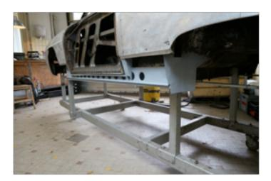
During the renewal of the sills an extra stiffening plate was welded in along the full length of the cars sides. To this much stronger construction the lower ends of the A and B pillar were welded thus prohibiting the body from further flex.
