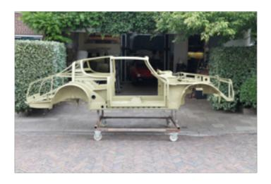
With the car now structurally sound it was safe to remove the complete aluminum skin and send the car to the sandblaster whose work revealed some extra corrosion damage in the rear boot sections floor. Complete sections had to be reproduced and welded in. Now correct in all detail the steel structure was painted in 3 layers with the top one in black.
