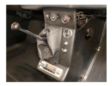
In the center console a period correct UHF radio – connected to the one speaker under the rear window - is installed but she will only connect you to the howl of the
