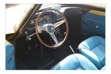
The original Sport interior was newly clothed using the correct shade of blue leather on all seats and the side panelling. For the door panels the originally used pressed wood was replaced by moist resistant black plastic of the same thickness. Onto them all the original ornaments and brightwork were mounted.
